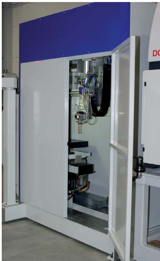
Service accessibility through service door at the side. Optimum access to all components on the interior of the system.
