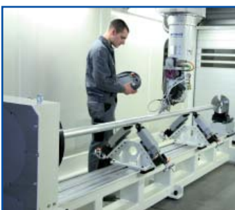
Contour mapping with teach unit
