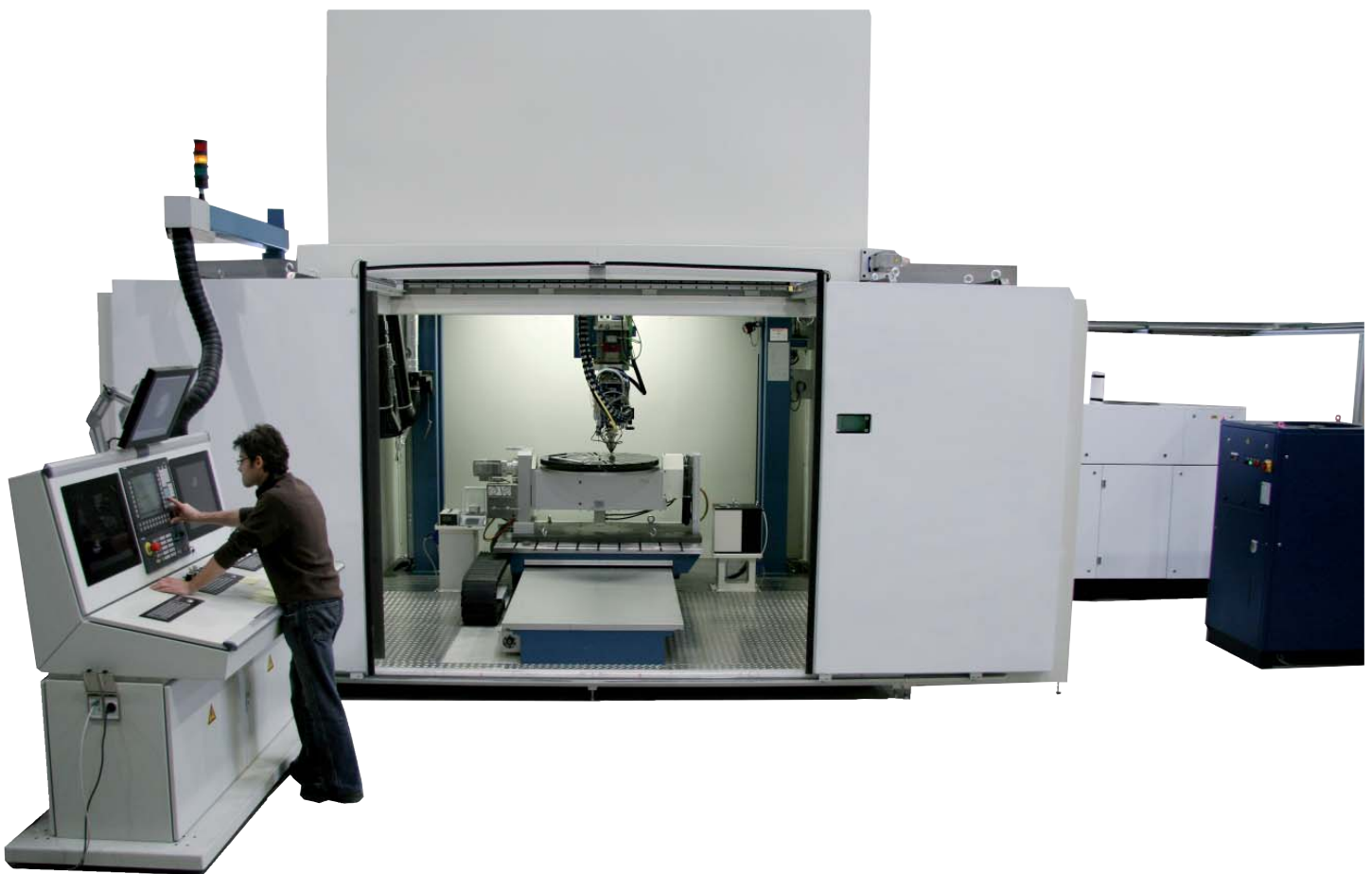
Machining head with rotary/tilt table
