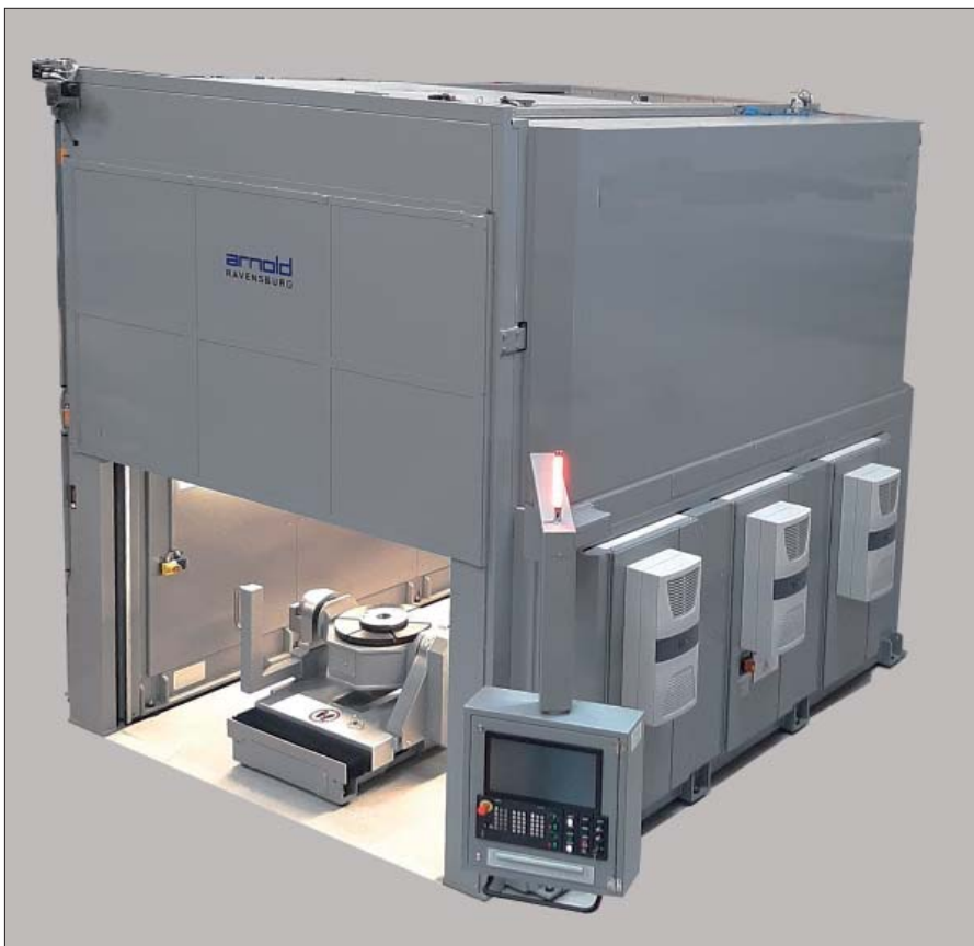
Gantry for powder and wire application welding as well as laser cutting
